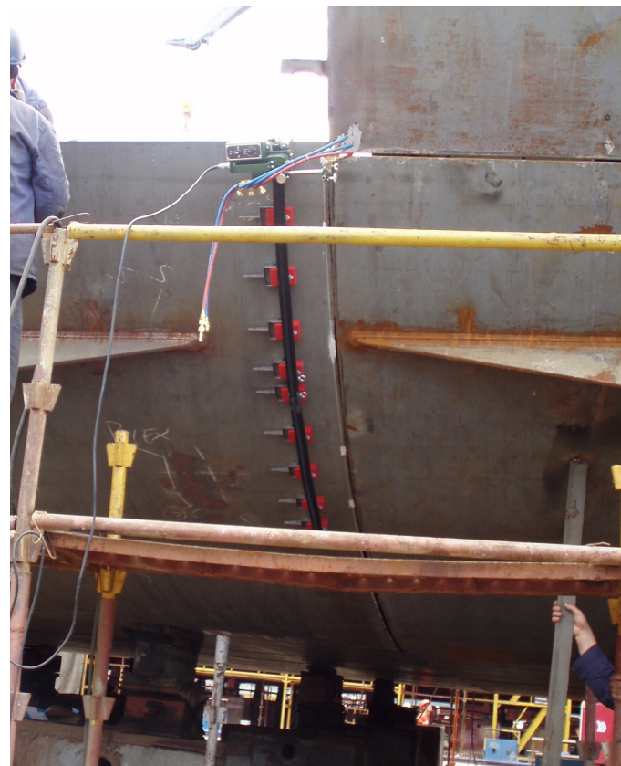
Welding preparation performed with 2D rail
