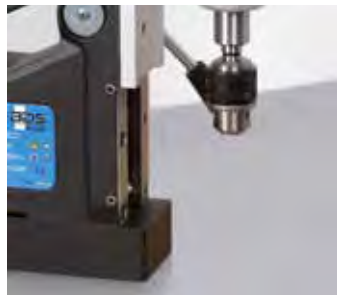
2. Insert drill chuck in MT arbor.
