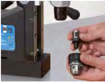
1. Connect adapter to drill chuck.
