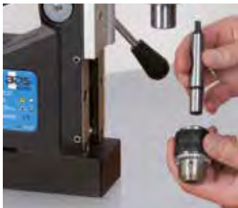
1. Connect taper drift to drill chuck.
