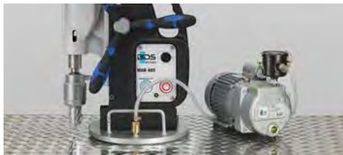
Vacuum plate for smooth corrugated sheet metal/gussets
