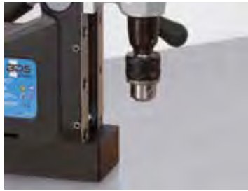
2. Insert drill chuck into the direct arbor.
